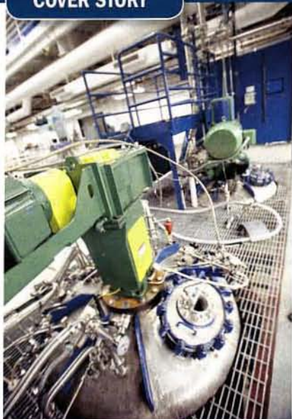
SCALING UP: Genomatica is producing bio-BDO in 3,000-liter fermentation tanks.
