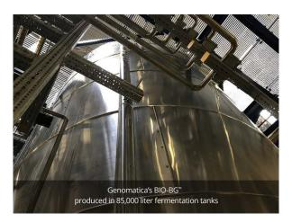
Genomatica has begun to produce Bio-BG™ butylene glycol in large scale, 85,000 liter fermentation tanks at EW Biotech in Leuna, Germany.
