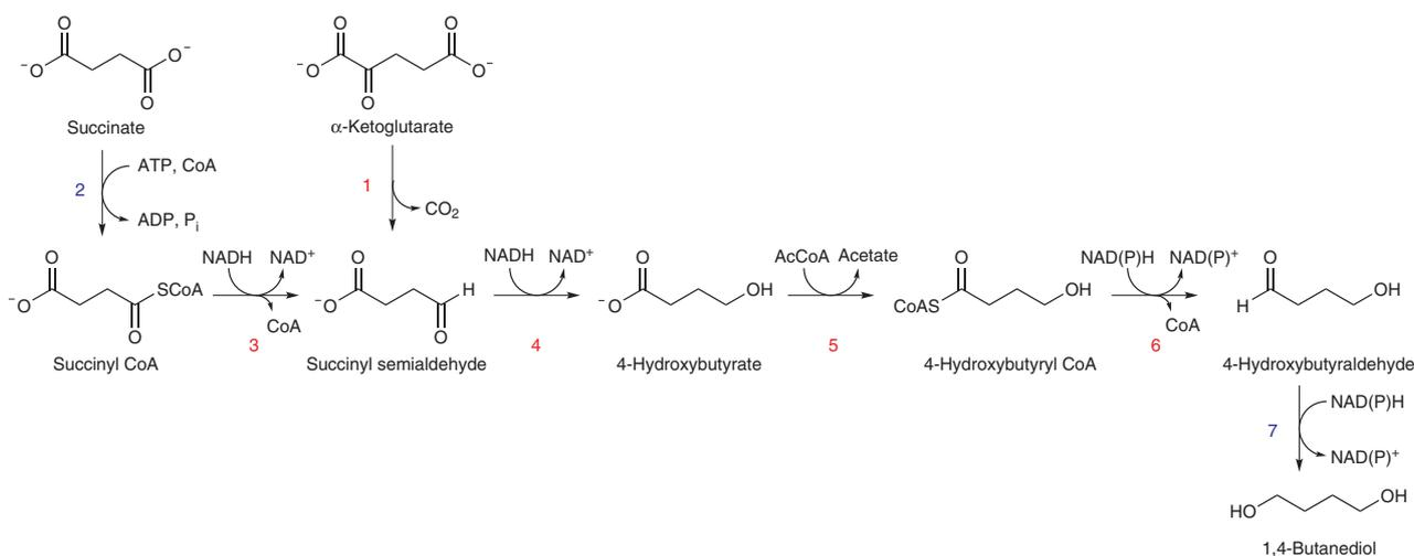
**Scheme 1 | BDO biosynthetic pathways introduced into *E. coli*.** Enzymes for each numbered step are as follows: (1) 2-oxoglutarate decarboxylase; (2) succinyl-CoA synthetase; (3) CoA-dependent succinate semialdehyde dehydrogenase; (4) 4-hydroxybutyrate dehydrogenase; (5) 4-hydroxybutyryl-CoA transferase; (6) 4-hydroxybutyryl-CoA reductase; (7) alcohol dehydrogenase. Steps 2 and 7 occur naturally in *E. coli*, whereas the others are encoded by heterologous genes introduced in this work.
