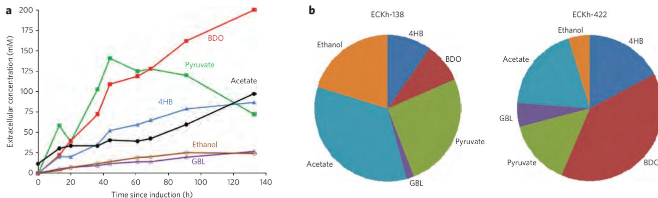
**Figure 5 | Production of BDO from glucose in 2-l fed-batch fermentation using the OptKnock strain ECKh-422.** The host was transformed with plasmids pZS\*13S-sucCD-sucD-4hbd/sucA and pZE23S-025B-34. (a) Fermentation profile. Extracellular concentrations are in fermentation broth. (b) Comparison of product profile at the end of this fermentation run (right) with that from a fermentation with ECKh-138 (left).
